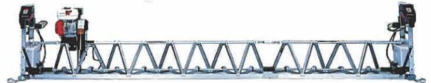
Truss Paver Screed
